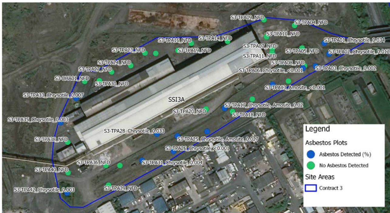
SSI3A Figure 6: Summary of Asbestos Testing
